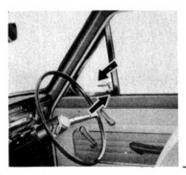
To open the ventilator, push the button. Turn the lever forward and move the ventilator out to the desired position.
