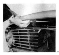
Pull the hood lock handle located at the lower right-hand side of the instrument panel, and then the safety catch, located under the center edge of the hood, must be pushed up to completely release the hood.
