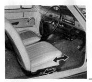
By pushing the adjusting lever backward you can move it forward and backward within the range of 5.5 in. (140 mm), with eight set positions.
